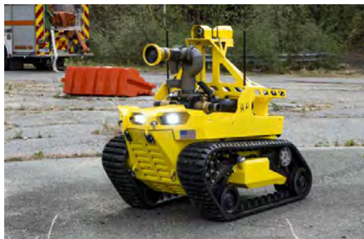
Figure 2 – Thermite: Robotic Fire Fighter
